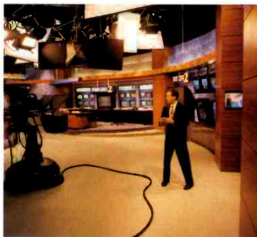
Sony camera is mounted on a robotic pedestal.
